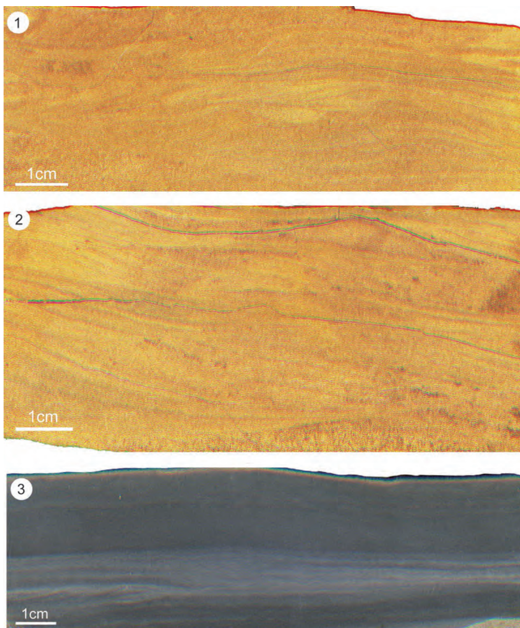
Fig. 35. Vertical cross sections of sandstone in the upper part of the Bac Thuy Formation. 1–2, Very fine siliciclastic sandstone contains climbing-ripple lamination from NT01. 3, Thin calcareous turbidite characterized by Tc and Td divisions is embedded in thick hemipelagic mudstone at KC02-15.
