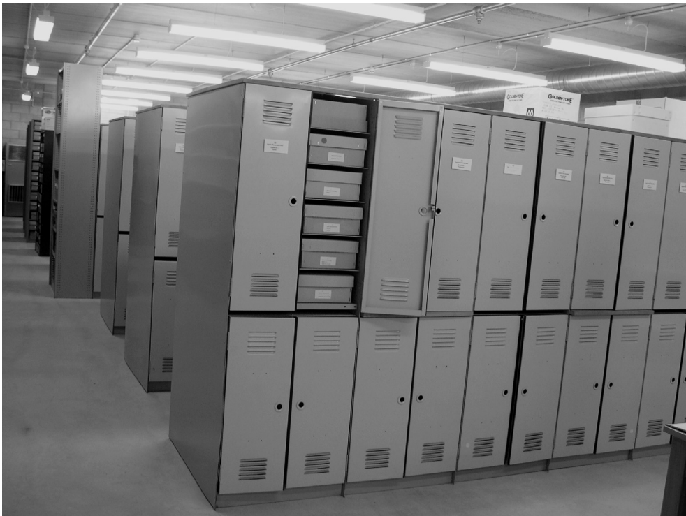
Fig. 6. The collection vault of the New Zealand Fungal Herbarium (PDD). The vault is climate controlled (18°C, RH 50%) and has a gas-flood fire control system. To assist with insect control, all collections are frozen for one week before they are taken into the vault.
