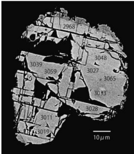
Fig. 8. The oldest monazite grain found from Sibuyan. Numbers in the grain are age shown as Ma. Obtained age is 3036 \pm 17 Ma.
