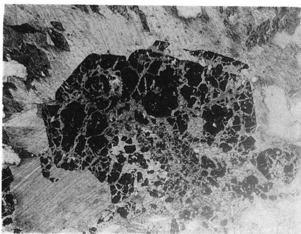
Fig. 2. Photomicrograph of a magnetite grain embedded in calcite. It is partially pseudomorphed by minutely developed network of chamosite. One polar. Field view 3.3 \times 4.75 mm.
