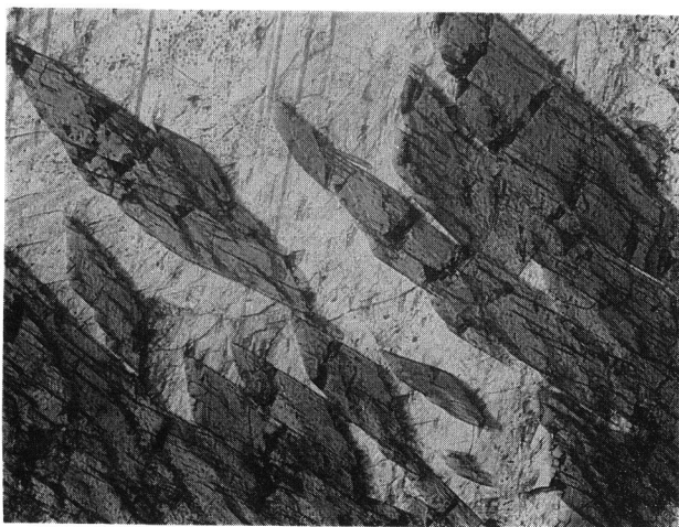
Fig. 1. Photomicrograph of isolated prismatic forms of hastingsitic hornblende embedded within larger calcite grains. One polar. Field view: 0.53 \times 0.76 mm.
