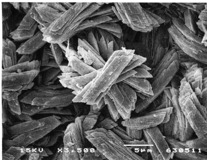
Fig. 1. Electron microscope images of gyroidal aggregates of idiormorphs of turquoise demonstrating the parallelogram-shaped outline and the perfect cleavage. A bar indicates 5 \mu\text{m} .
