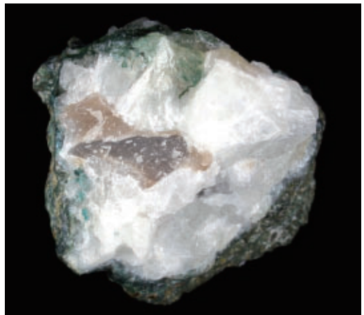
Fig. 4. “Okenite” aggregate fills cavity of apophyllite crystals in amygdule. Specimen is approximately 30 mm in width.
