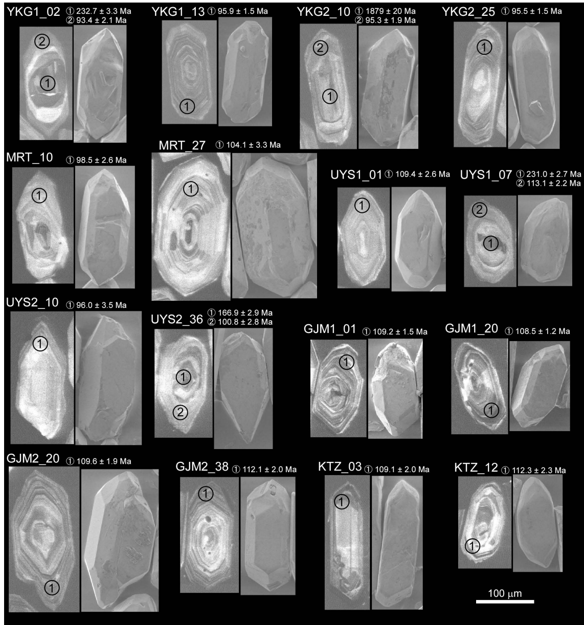
Fig. 3. Morphological secondary electron (SE) images before cement in resin and cathodoluminescence (CL) images of analyzing section of typical zircon grains from the samples. Circles on the images indicated analyzed spots by LA-ICP-MS. Spot diameter is 25 \mu m approx.
