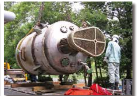
大型資料の搬入：塩化ビニル重合器 Installation of a large object to the store house: Polymerization reactor of vinyl chloride
